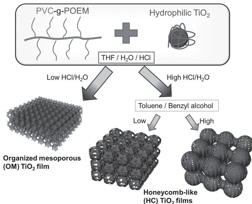
Figure 1. Schematic of the preparation of OM and HC series \text{TiO}_2 films using PVC-g-POEM graft copolymer and hydrophilically preformed \text{TiO}_2 nanocrystals.
